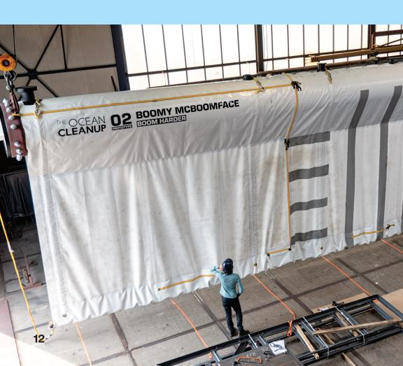
A three-metre screen hangs down from the floater and collects the smaller pieces of plastic that are under the water. As it is a screen and not a net, fish and other marine animals don't get trapped in it. They can just swim under it.
