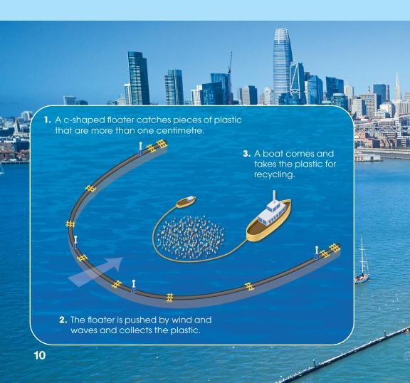
A team of one hundred scientists and engineers studied the problem. Their solution was to create a giant c-shaped 'floater', six hundred metres long, that would float on the surface of the ocean and collect plastic rubbish. When there was enough plastic, a boat would come to take the plastic back to land. The plastic would then be recycled and used to make products like phones, plastic chairs or sunglasses.
